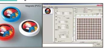
Total printing time (White printing+Color printing): 22 min., 24 sec. Size: 29 mm dia., 1,200 x 1,200 dpi, 16 pass Hi-mode Width 600 mm x feeding direction 500 mm, with 168 units imposed.
