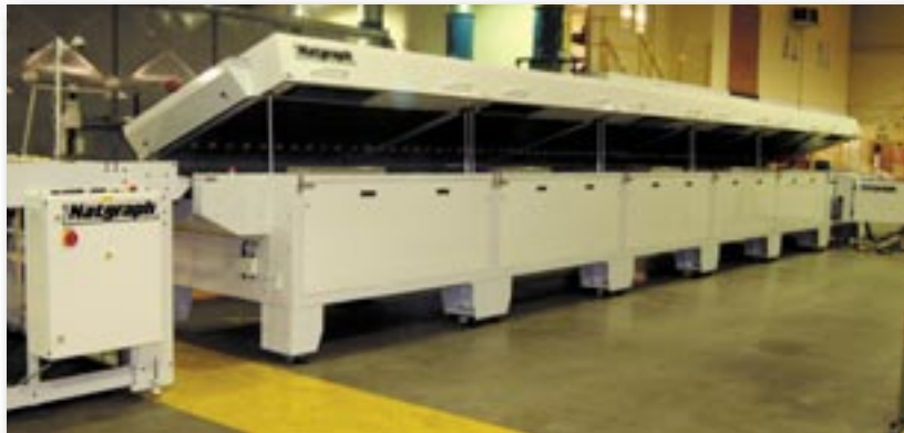
4 Heating and 2 Cooling modules
