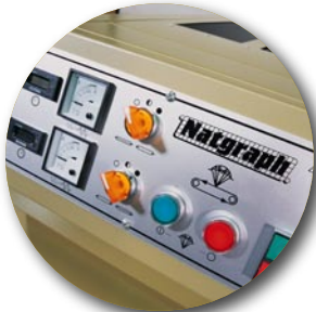
UV Bridge Control Panel
