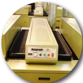
UV Bridging Modules Installed
