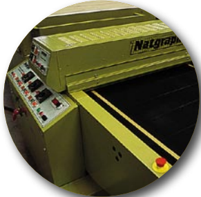
UV Bridge on Air Force Dryer
