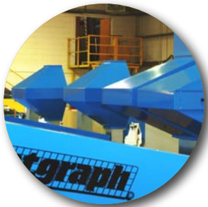
Inlet filter stacks
