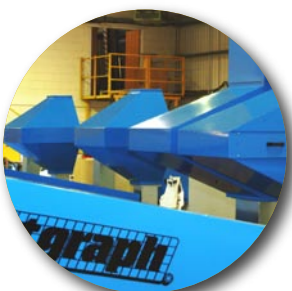
Inlet Air Filter Stacks
